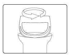
(2) Unscrew and remove the pump by turning the handle in an anti-clockwise direction.
