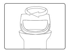
4 Screw the pump handle back into position by turning the handle in a clockwise direction. Ensure all fittings are tightened before proceeding.
