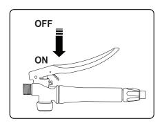
Spray the desired area by holding down the trigger on the nozzle. The trigger can be locked for continual spraying.
