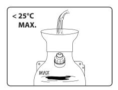
(3) Fill the bottle with liquid to the desired level. Do not exceed the maximum capacity level marked on the bottle.
