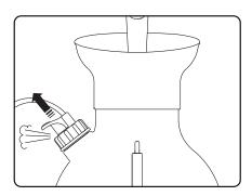
(1) Before filling, release any pressure built up within the bottle by lifting the safety valve.
