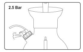
9 Ensure that pressure is released and that all sprayer components are rinsed thoroughly with water after use. This can be achieved by filling the bottle with clean water, pressurising and then emptying via the nozzle. Clean after every use and do not store liquids in the unit.
