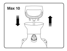
5 Pressurise the bottle by pumping the lever up to 10 times. Do not over pressure.
